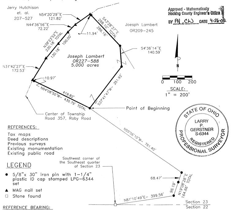
East line of Section 22 as South 0 degrees 13 minutes 23 seconds West. Bearings are based upon an assumed meridian and are to denote angles only.
