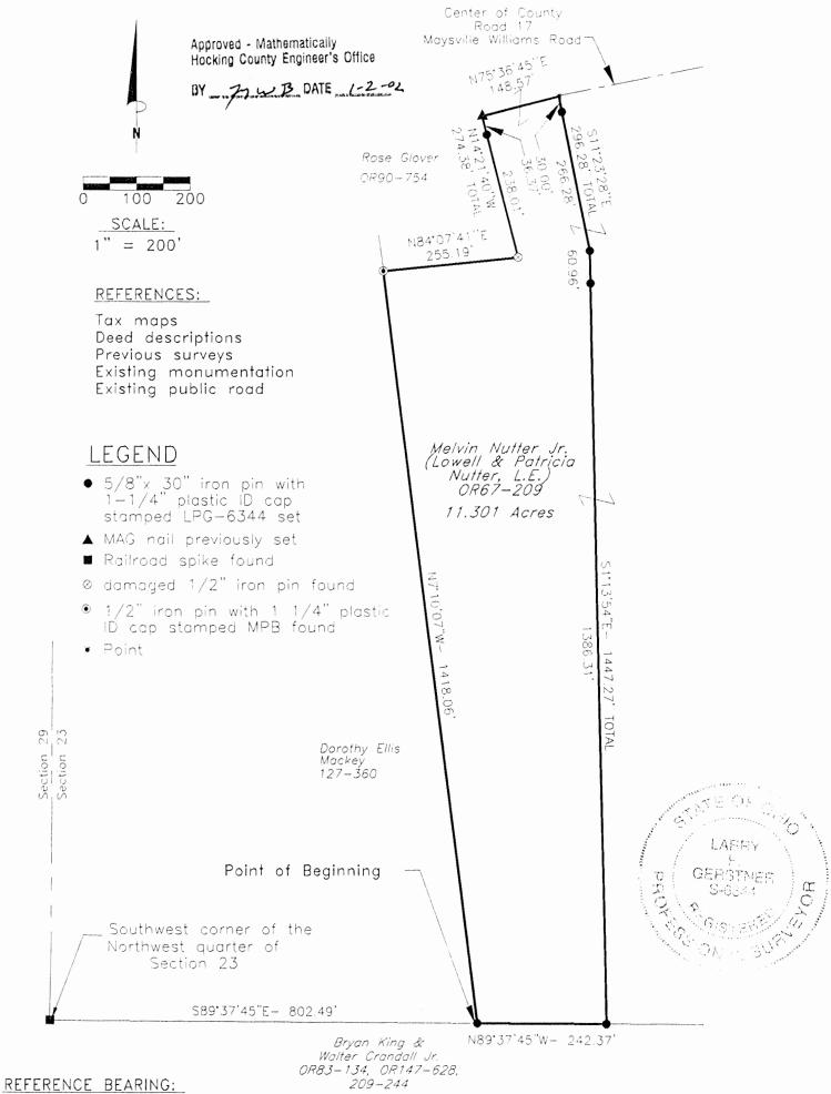
North line of Section 23 as South 89 degrees 46 minutes 43 seconds East. Bearings are based upon an assumed meridian and are to denote angles only.
