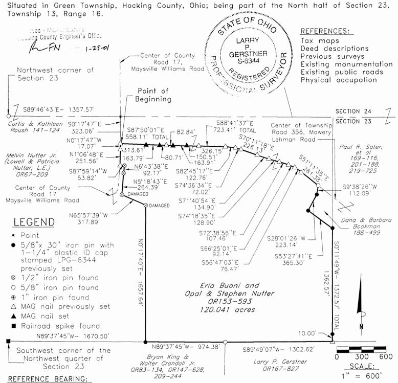
North line of Section 23 as South 89 degrees 46 minutes 43 seconds East. Bearings are based upon an assumed meridian and are to denote angles only.
