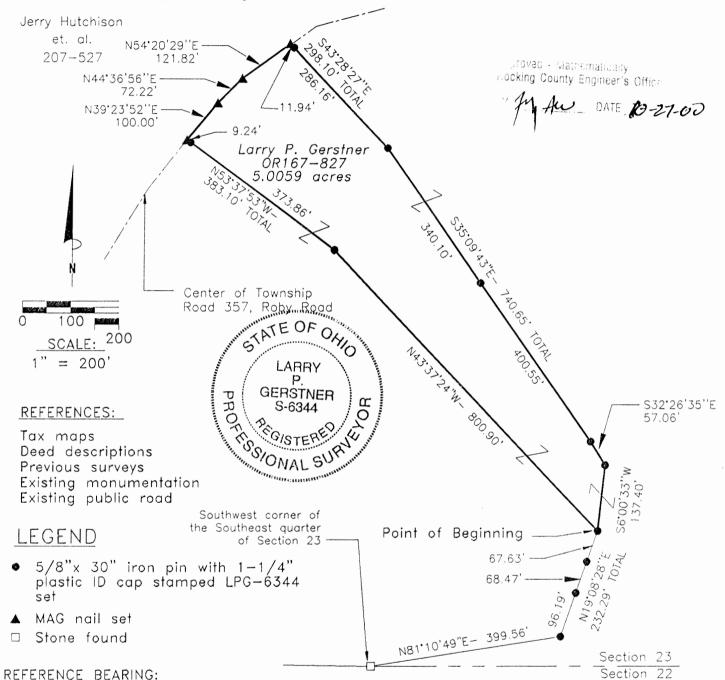
East line of Section 22 as South 0 degrees 13 minutes 23 seconds West. Bearings are based upon an assumed meridian and are to denote angles only.
