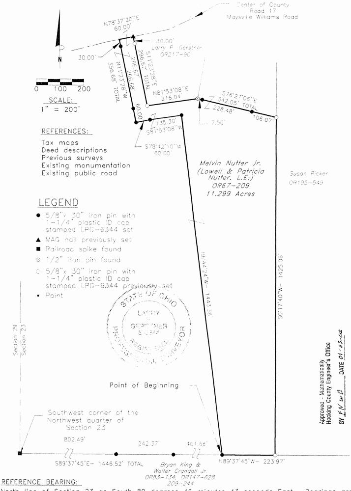
North line of Section 23 as South 89 degrees 46 minutes 43 seconds East. Bearings are based upon an assumed meridian and are to denote angles only.
