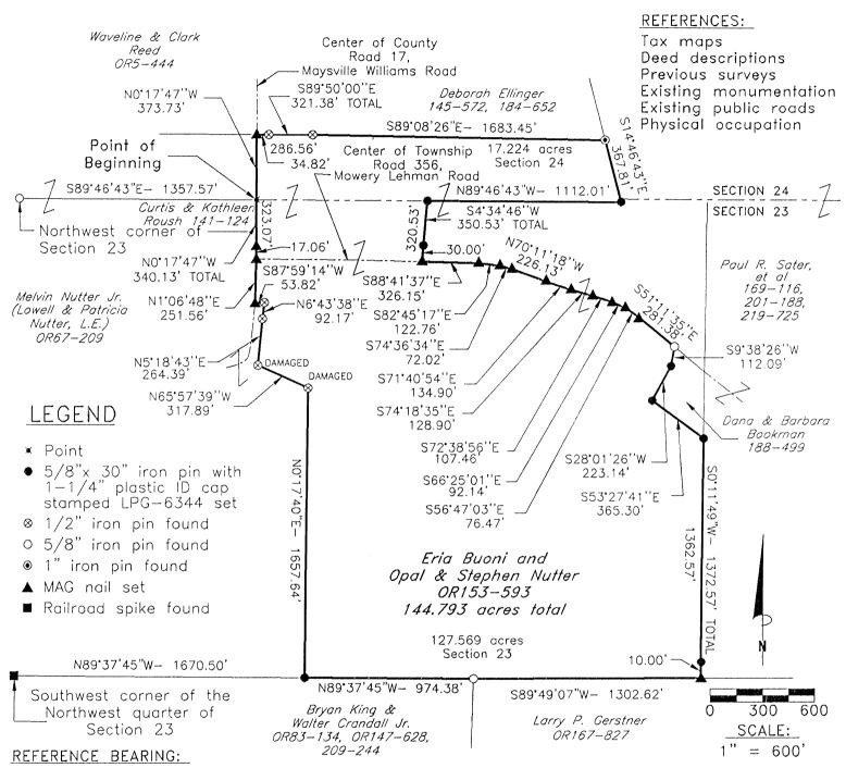
North line of Section 23 as South 89 degrees 46 minutes 43 seconds East. based upon an assumed meridian and are to denote angles only.
