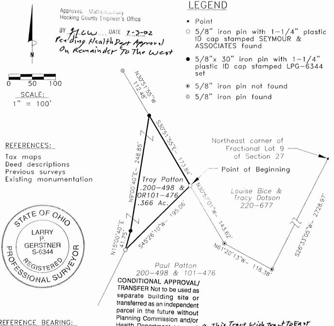
North line of Section 27 as North 89 degrees 32 minutes 40 seconds West. Bearings are based upon an assumed meridian and are to denote angles only.
