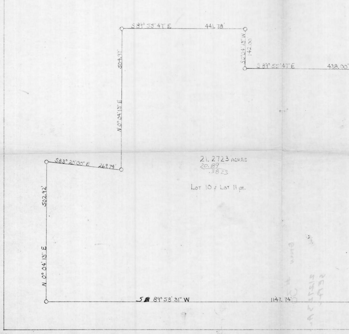
O-IRON PIN 832.82 D-STONE SCALE 1"=100' DATE 5-21-76 BEING Lot 10 + Lot 11 pr., SEC. 36, T-13-N R-16-W, GREEN TWP. Hocking Co., Bhio Surveyed & planed for Richard S. Downhey Sr. by GEORGE F. SEYMOUR & ASSOCIATES P.O. Box 26 LOGAN, Ohio S 0° 04' 13" W REGISTERED SURVEYOR #6044 APPROVED HOCKING COUNTY ENGINEER'S OFFICE DATE BY\_ SE CORNER 5 897.76 - 09 SEC. 36 T-13-N, R-16-W GREEN TWP.
