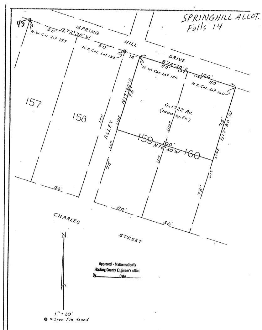
Map Showing Survey of 0.1722 Acre Situate: 996 Spring Hill Drive, Logan, Ohio Being a part of Section 14, Falls Twp., Hocking County, Ohio, and being the North half of Lots 159 and 160 of of the Spring Hill Addition, recorded in Plat Book No. "B", Page 50, Hocking County Records.
