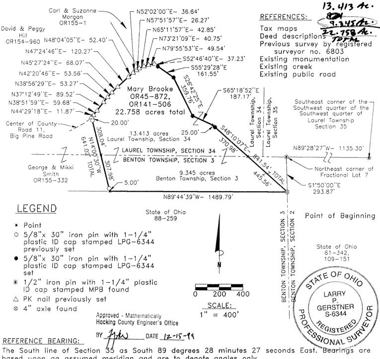
The South line of Section 35 as South 89 degrees 28 minutes 27 seconds East. Bearings are based upon an assumed meridian and are to denote angles only.
