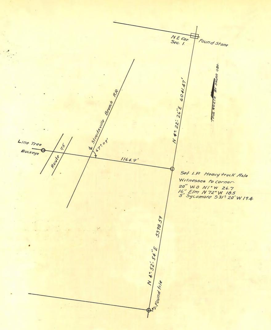
I certify that I have Placed an iron pin at the South East Corner Section I Folls two. in accordance with an old Survey found in Vol. 123 Straitsville Branch of the C.&.O. R.R. under date of 1879. Ond filed in office of Valuation Eng. C.& O. R.R. Spahr Bldg. Columbus, Ohio.
