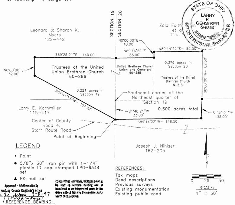
The East line of the Northeast quarter of Section 19 as North 0 degrees 00 minutes 00 seconds East. Bearings are based upon an assumed meridian and are to denote angles only.
