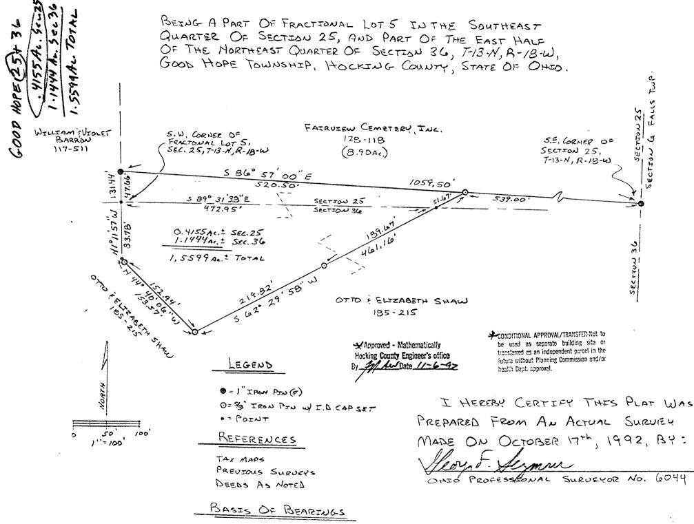
THE BEARINGS USED WERE DERIVED FROM A PREVIOUS SURVEY AND ARE TO BE USED FOR THE DETERMINATION OF ANGLES ONLY.
