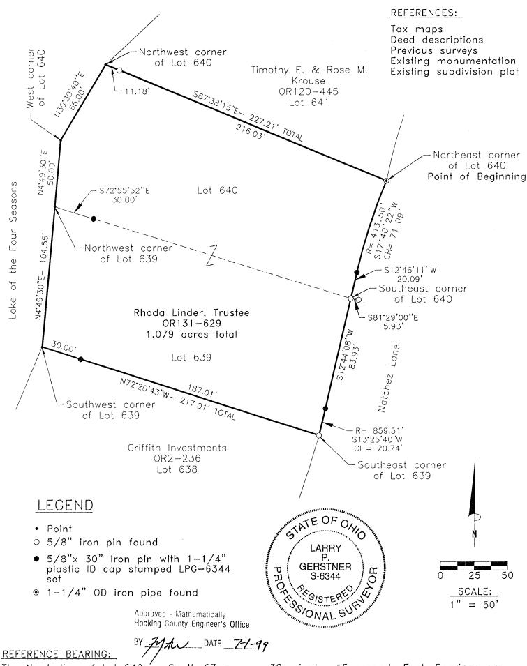
The North line of Lot 640 as South 67 degrees 38 minutes 15 seconds East. Bearings are based upon an assumed meridian and are to denote angles only.
