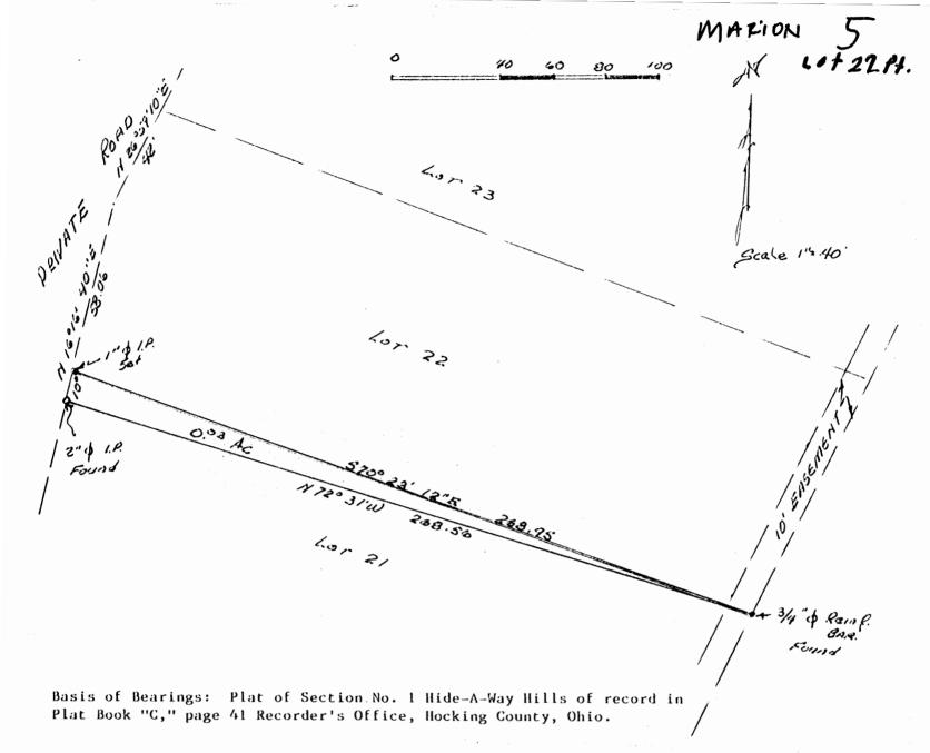
Situated in the Township of Marion, County of Hocking, State of Ohio and being a part of Lot No. 22 of HIDE-A-WAY HILLS SECTION NO. 1 as the same is numbered and delineated upon the recorded plat thereof, of record in Plat Book C, Page 41, Recorder's Office, Hocking County, Ohio bounded and described as follows:
