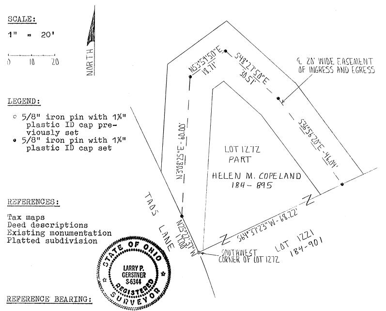
The plat of Sections 45 of Hide-A-Way Hills making the Northeast line of Lot 1273 of Hide-A-Way Hills as South 43 degrees 49 minutes 46 seconds East.
