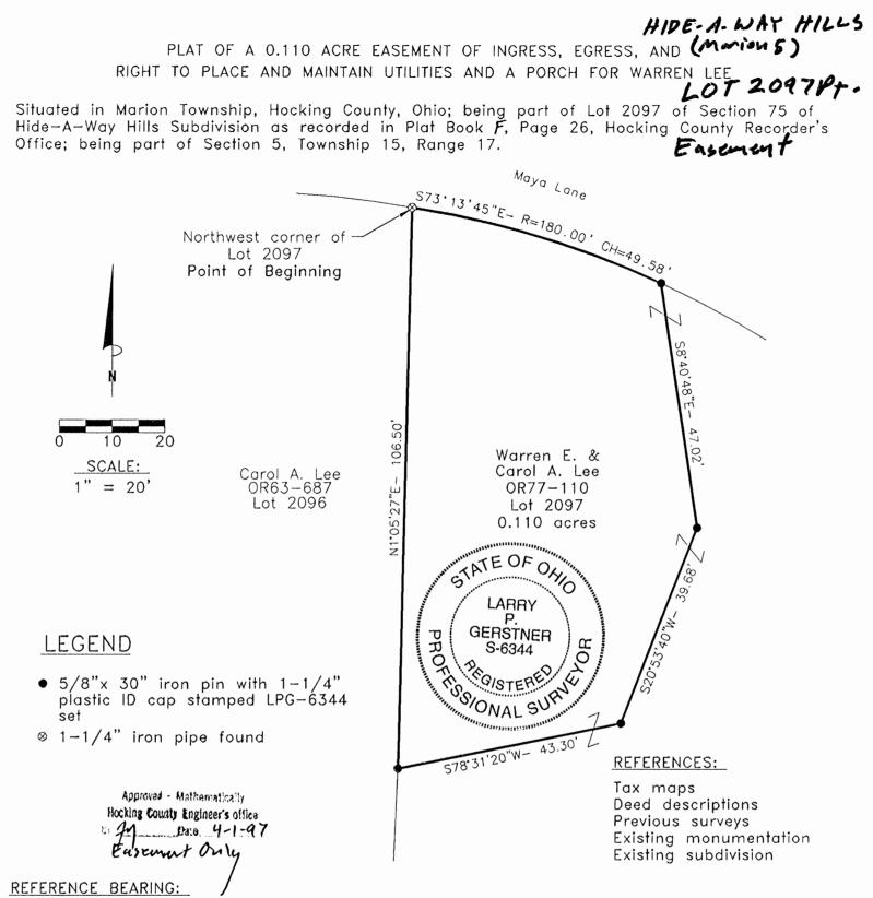
The Plat of Lot 2097 making the West line North 1 degree 05 minutes 27 seconds East. Bearings are based upon an assumed meridian and are to denote angles only.
