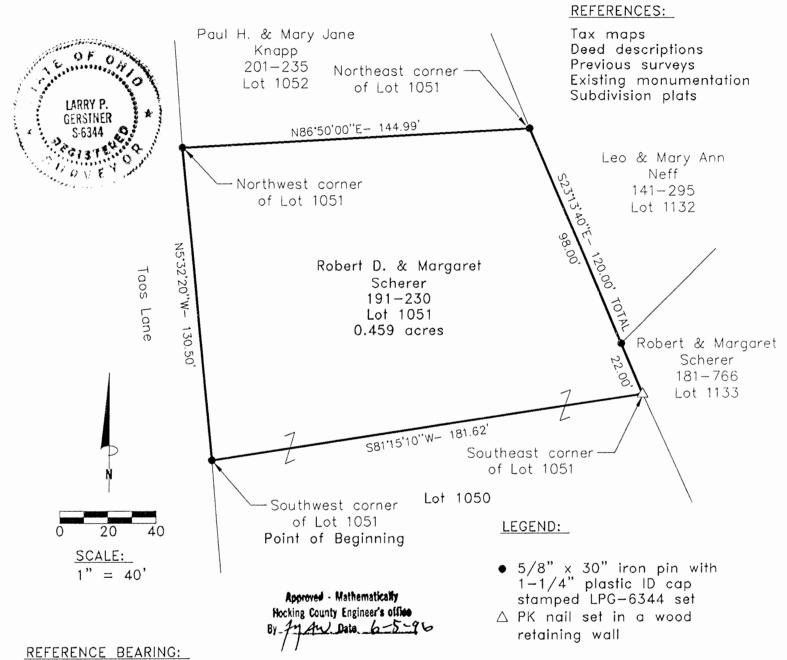
The recorded plat of Section 38 of Hide-A-Way Hills. Bearings are based upon an assumed meridian and are to denote angles only.
