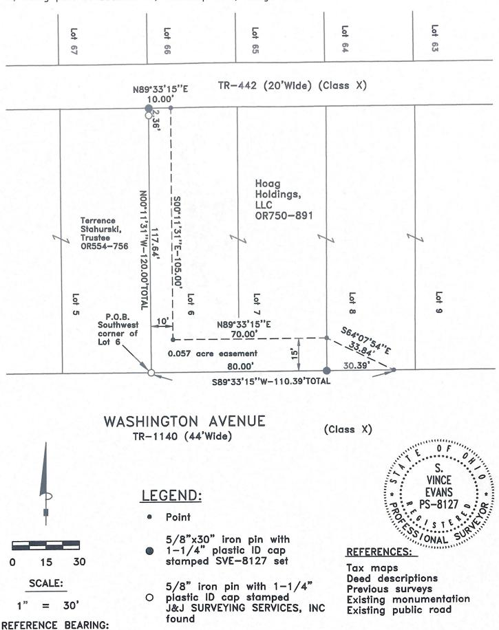
The north line of Washington Avenue as South 89 degrees 33 minutes 15 seconds West. Bearings are based upon an assumed meridian and are to denote angles only.
