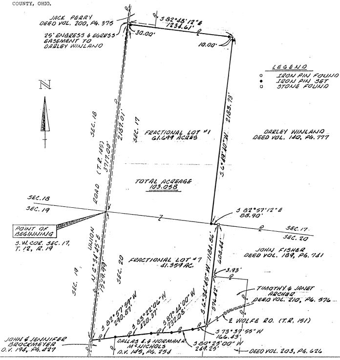
The bearing system for this plat is based on the east line of Fractional Lot No. 7, Section 20, Township 12, Range 19 as being S 6° 34' 45" W. I hereby certify that this plat was prepared from an actual field survey of the premises in <u>January</u> of 1991 and from existing public records and that said plat correctly defines the limits of the parcel shown hereon.
