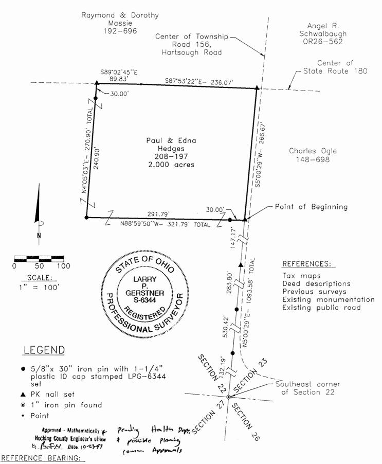
The South line of Section 22 as North 85 degrees 54 minutes 57 seconds West. Bearings are based upon an assumed meridian and are to denote angles only.
