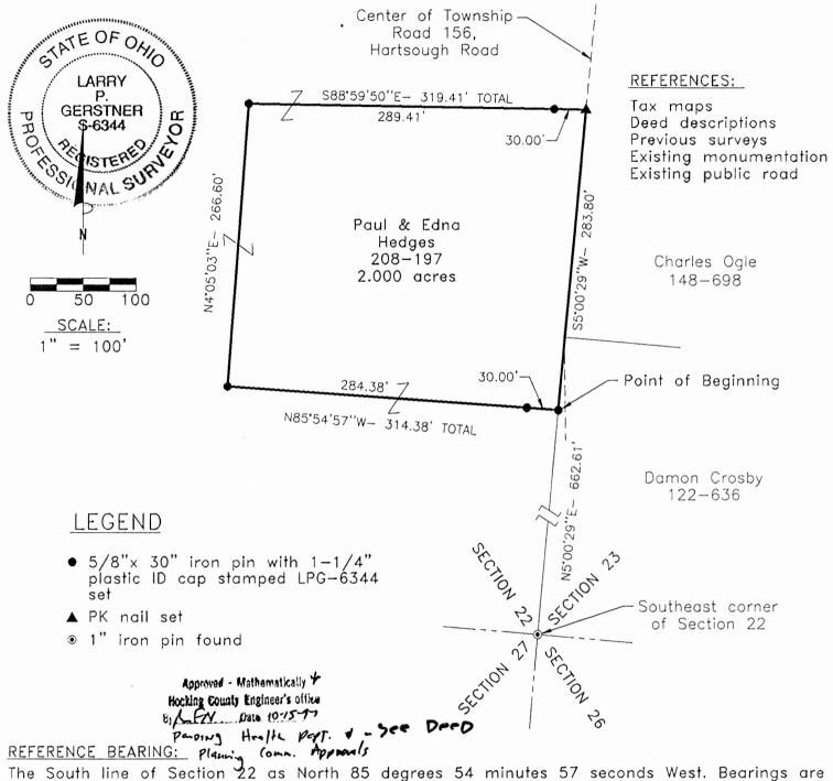
The South line of Section 22 as North 85 degrees 54 minutes 57 seconds West. Bearings are based upon an assumed meridian and are to denote angles only.
