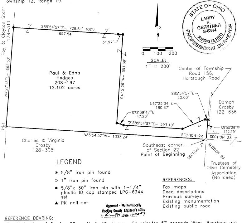
The South line of Section 22 as North 85 degrees 54 minutes 57 seconds West. Bearings are based upon an assumed meridian and are to denote angles only.
