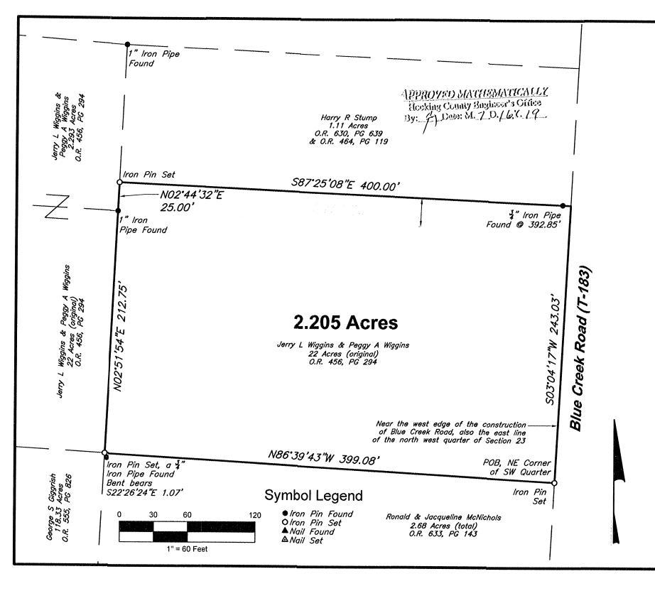
IRON PINS SET ARE 5/8" DIAMETER X 30" LONG REBAR WITH RED PLASTIC CAP STAMPED "H&S 8592" ALL IRON PINS SHOWN AS FOUND ARE IN GOOD CONDITION UNLESS NOTED OTHERWISE.
