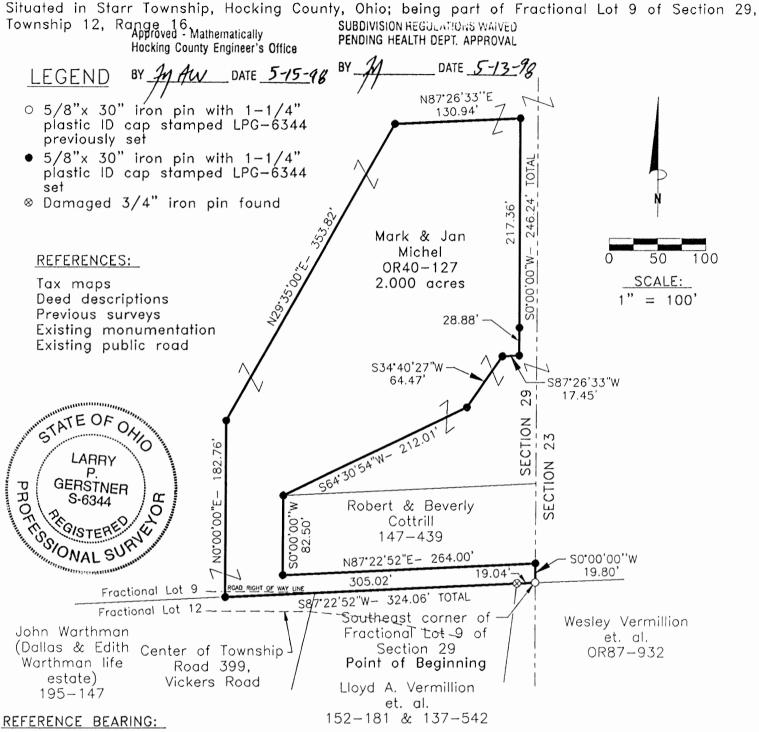
The East line of Section 29 as South 0 degrees 00 minutes 00 seconds West. Bearings are based upon an assumed meridian and are to denote angles only.
