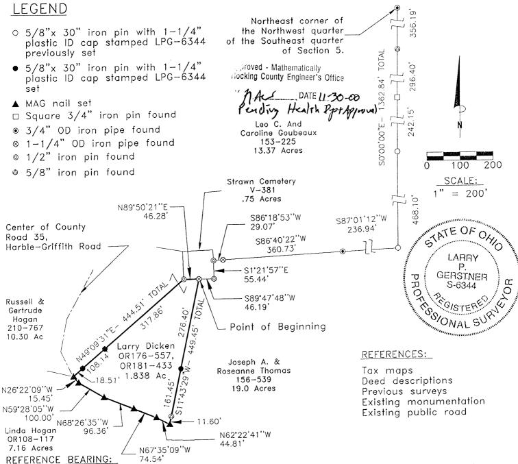
East line of the Northwest quarter of the Southeast quarter of Section 5 as South 0 degrees 00 minutes 00 seconds East. Bearings are based upon an assumed meridian and are to denote angles only.
