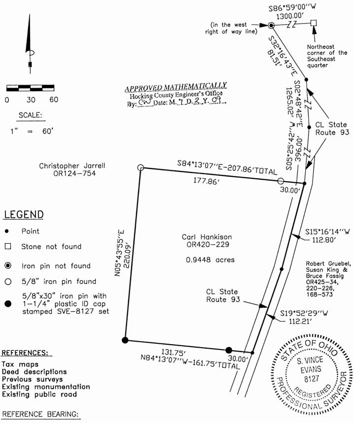
The north line of a 0.9448 acre tract as South 84 degrees 13 minutes 07 seconds East. Bearings are based upon an assumed meridian and are to denote angles only.
