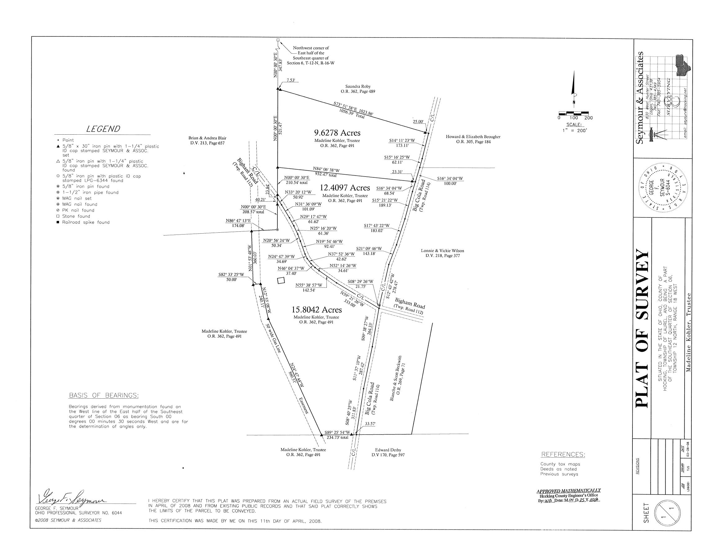
Beginning at 5/8" X 30" iron pin with a 1 1/4" plastic identification cap set on the West line of the East half of the Southeast quarter of Section 6, from which a stone found on the Northwest corner of the East half of the Southeast quarter bears North 00 degrees 00 minutes 30 East a distance of 347.83 feet;
