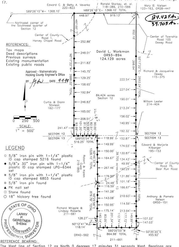
The West line of Section 12 as North 0 degrees 17 minutes 31 seconds West. Bearings are based upon an assumed meridian and are to denote angles only.
