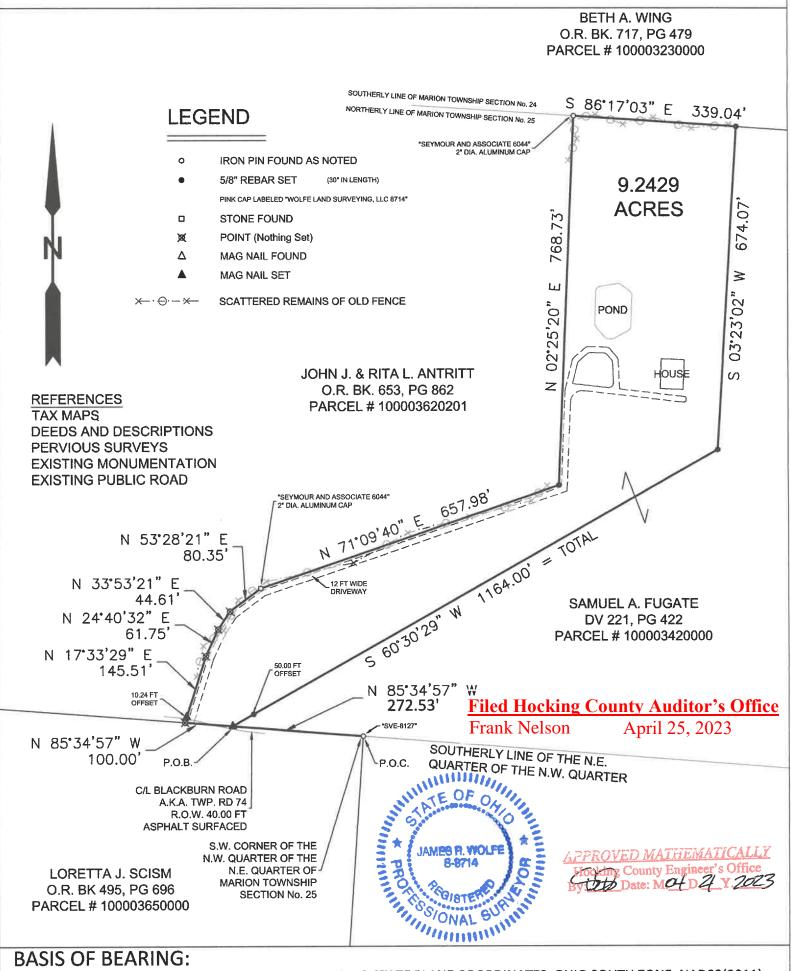
THE BASIS OF BEARING ARE BASED ON GRID NORTH, OHIO STATE PLANE COORDINATES, OHIO SOUTH ZONE, NAD83(2011) AS BASES UPON GEODETIC OBSERVATIONS USING THE OHIO VRS NETWORK AND ARE USED TO DENOTE ANGLES ONLY.
