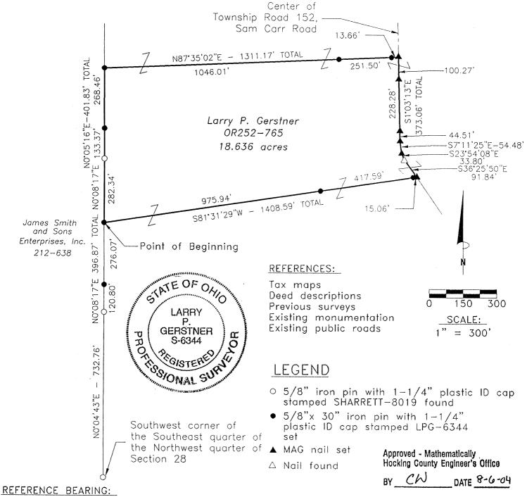
East line of Section 28 as South 0 degrees 00 minutes 00 seconds East. Bearings are based upon an assumed meridian and are to denote angles only.
