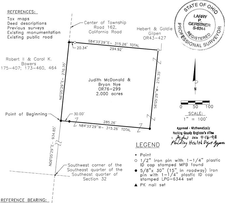
The East line of Section 32 as North 4 degrees 51 minutes 15 seconds East. Bearings are based upon an assumed meridian and are to denote angles only.
