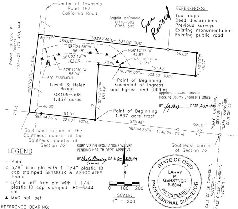
The South line of said Section 32 as North 83 degrees 44 minutes 36 seconds West. Bearings are based upon an assumed meridian and are to denote angles only.
